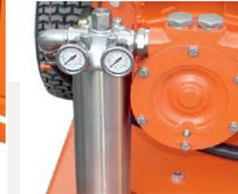
Stainless steel pump-head. Integrated cooling for plunger-seals.
