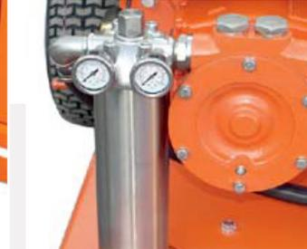
Stainless steel pump-head. Integrated cooling for plunger-seals.
