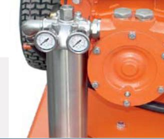
Stainless steel pump-head. Integrated cooling for plunger-seals.
