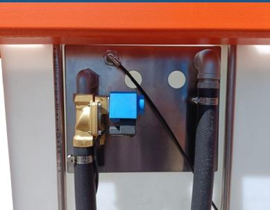
Solenoid valve for water supply
