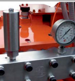
Stainless steel pump-head. Integrated cooling for plunger-seals.
