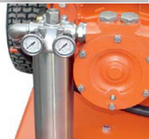
Integrated booster pump & filter system.
